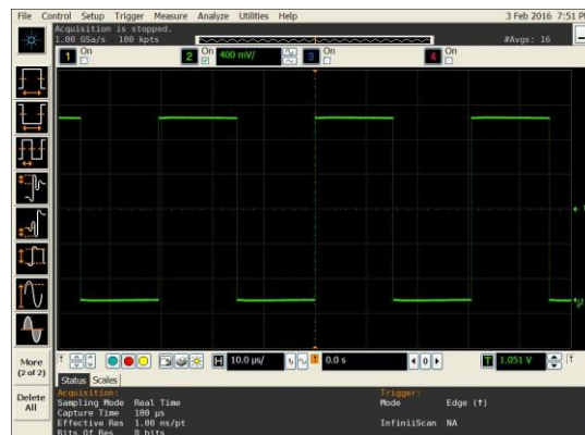
Figure 9. LVCMOS Output Swing
